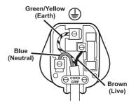
Ensure that the outer sheath of the cable is firmly held by the clamp
